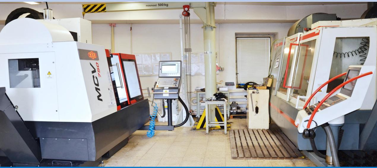
Machining of products is made by CNC machining automat MCV 1000 SPEED and MCV 750 SPEED acc to customer's drawings.
