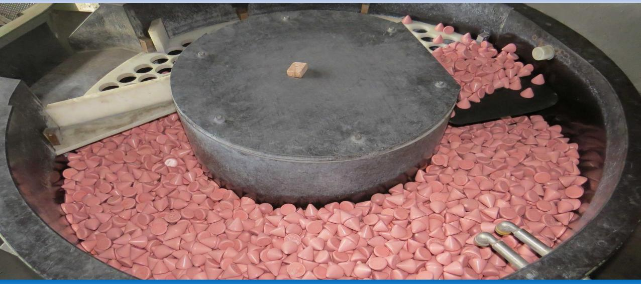
We are able to solve a huge range of technological requierements by tumbling technology. For instance treatment of sharp edges and burrs, polishing and smoothing of surface, degreasing, cleaning and removing of rust.
