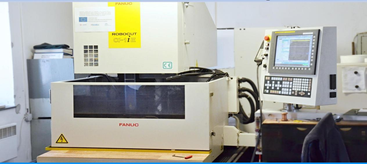
KOMAS is able to cut products by electroerosive wire cutting technology CNC FANUC Robocut equipment.
