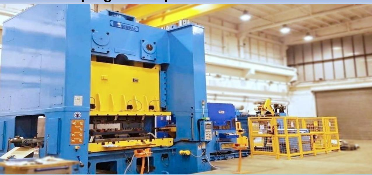
Pressing force of mechanical progressive press SIMPAC is 500t, stroke per minutes (SPM) 20-40, adjustable height of the tool 250mm, slide dimension 3.200x1400mm, Material: steel / Al, Material thickness: 0.6-6mm, Coil width: 200-600mm, Max. coil weight 5t
