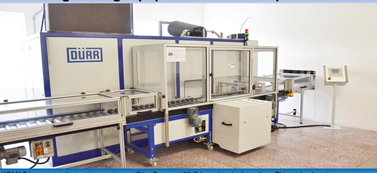
KOMAS has a new degreasing equipment Dürr Compact 80 C based on hydrocarbon. This technology is environmentally friendly, process of degreasing is vakuum closed.
