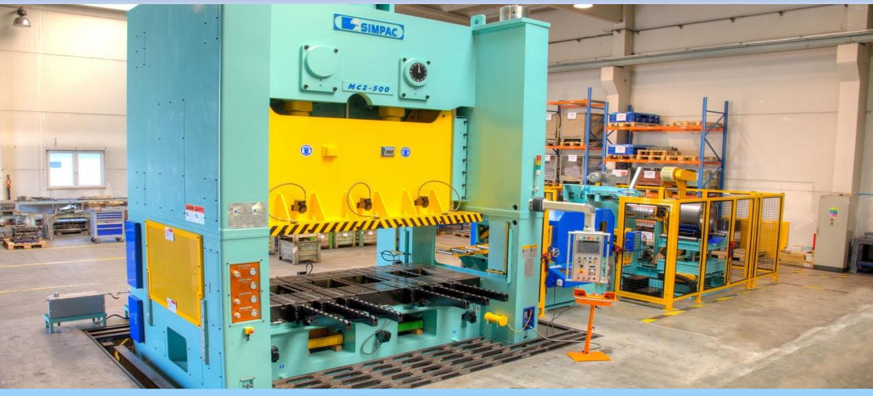
Pressing force of mechanical progressive press SIMPAC is 500t, stroke per minutes (SPM) 20-40, adjustable height of the tool 250mm, slide dimension 3.200x1400mm, Material: steel / Al, Material thickness: 0.6-6mm, Coil width: 200-600mm, Max. coil weight 5t
