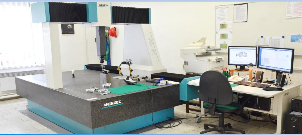
Measuring of products is realized by measuring equipment CNC 3D WENZEL LH 108. Measuring is made by KOMAS qualified .employees acc. to drawings or 3D model.
